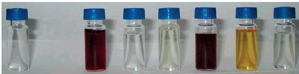
FIGURE 5. Colorimetric effect upon addition of TBA salts of anions (1 mM) to DMSO solutions of 1 ; left to right: 1 , F^- , Cl^- , H_2PO_4^- , HP_2O_7^{3-} , AcO^- , and NO_3^- .
